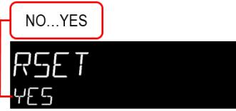
7. Press and hold the left knob (C) until the unit beeps to confirm the Reset setting.
