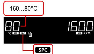
29. Press and hold the left knob (C) until the unit beeps and the heater indicator (M) illuminates.
